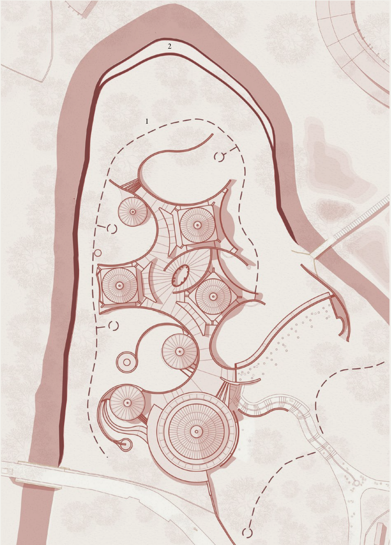
1. Extended land drain with water attenuation tanks 2. Reformed retention wall / riverbank to new height of 5m above sea level
